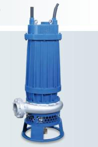
Head : 110 meters Capacity : upto 2500 m<sup>3</sup>/hr. RPM: 960/1450/2900 Motor : 0.75 to 222 kW Bearing : Double angular contact ball bearing and Deep groove ball bearing
