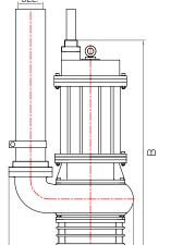
MANHOLE size nationwide is 600 mm and 540 mm, with its smart dimensions MBH MANHOLE pumps can be lowered in any manhole. All you need is a tripod or hydraulic crano
